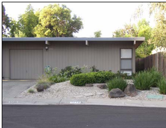
STYLE 8. Half-plex with vertical wood siding; wide fascia, overhang and exposed beams; tall vertical bedroom window; flat roof; front door on right side
