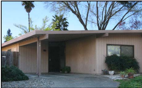
STYLE 5. Half-plex with vertical wood siding; wide fascia, overhang and exposed beams; horizontal bedroom window; carport; slightly sloped roofline
